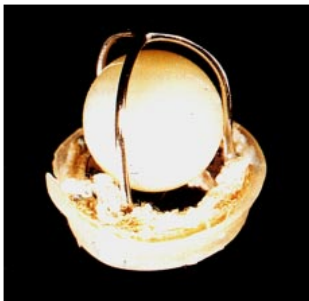
Figure 12. A caged-ball valve made in Mexico. This valve was recovered from a 17 year old patient who had it implanted at the age of 8 years. A new larger valve was implanted. Notice the excellent condition of this valve.
