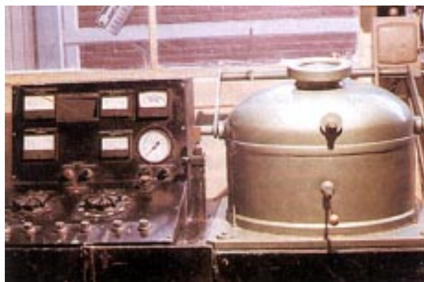
Figure 3. Vacuum metal chamber in which Stellite 21 metal is melted and cast to form the cage of prosthetic valves.
