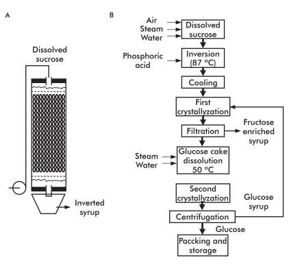
Figure 2. Steps of the technological process for the production of glucose and fructose syrup. A) Diagram of the enzymatic continuous reactor at laboratory scale. B) Acid hydrolysis.
