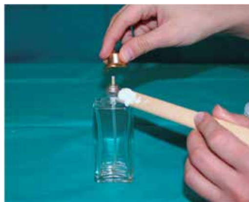
Figure 1. Preparation process of the container: a dosing valve is placed in the container's neck, which in then glued with an adhesive.
