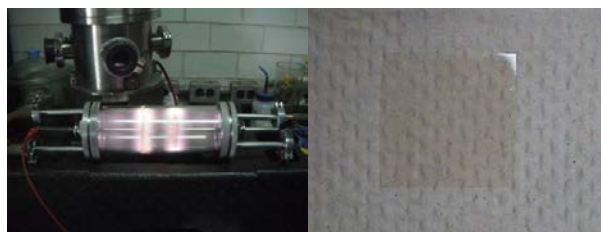
Figure 2. Left, plasma polymerization reactor. Right, material coated with polypyrrole by plasma.
