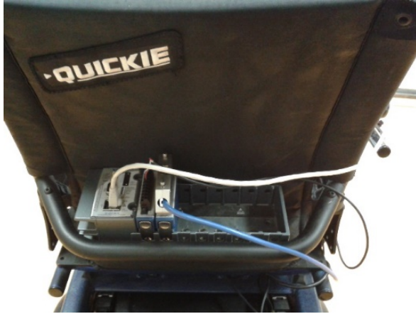
Figure 18. NI Compact-RIO installed for the real-time system.
