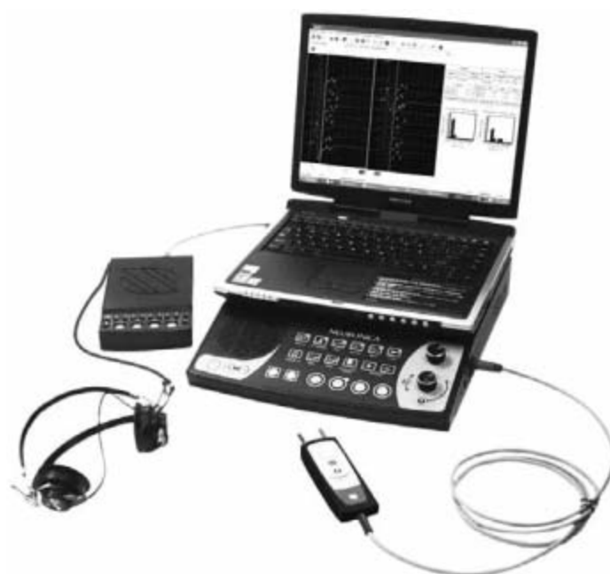
Figure 1: Neuronica. Cuban computerized system for neurophysiological studies such as evoked response testing and electromyography.
