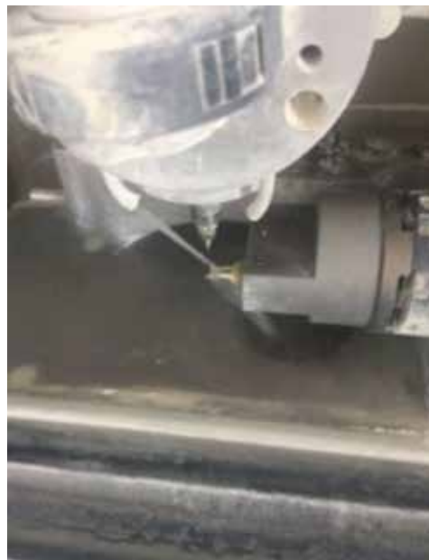
Figure 1. Closer view of dentin fragment being milled in CAD-CAM milling machine to generate dentin post.
