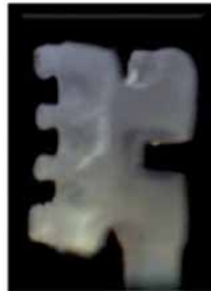
Figure 6. Retention rails on a polycarbonate bracket base.
