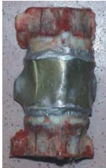
Figure 2. Test specimen made with photo elasticity varnish.
