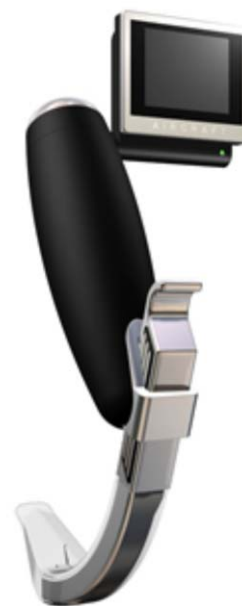
Figure 4. The McGrath Video Laryngoscope, featuring a position-adjustable «camera stick» covered by an easily-replaced transparent disposable sterile blade. A small LCD display located at the top of the laryngoscope handle can be adjusted to obtain the best view. The unit is powered with a single easily-replaced AA battery and features a single electronic control: an on/off switch located on the top of the unit.
